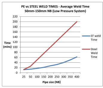
NOTE: The above weld times are based on actual on-site weld times and include pipe preparation and weld.
