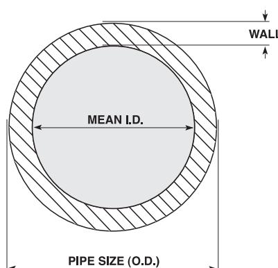
$$\text{SDR} = \text{OD} \div \text{WALL THICKNESS}$$
