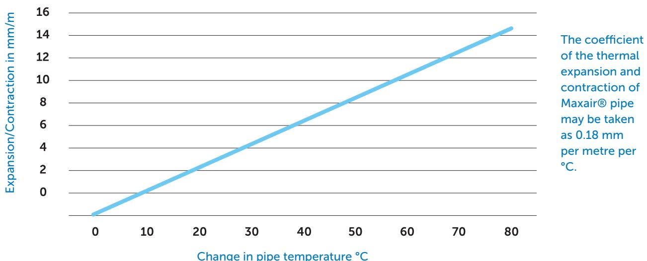
If pipework is to be subjected to thermal temperature change, expansion and contraction needs to be considered during installation. Generally movement can be absorbed on changes of direction, elbows, etc. but on longer lengths the recommended installation principles as set out on the following page should be adhered to.
