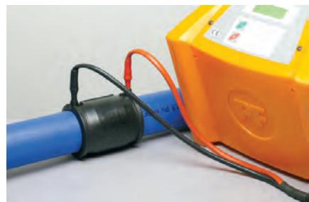
6. Connect welder leads onto fitting terminals (non specific). If using manual setting follow weld time as per label on fitting. Press start to commence weld cycle. Rising melt indicators confirm successful completion of weld. Remove leads and allow to cool without movement or strain on joint.
