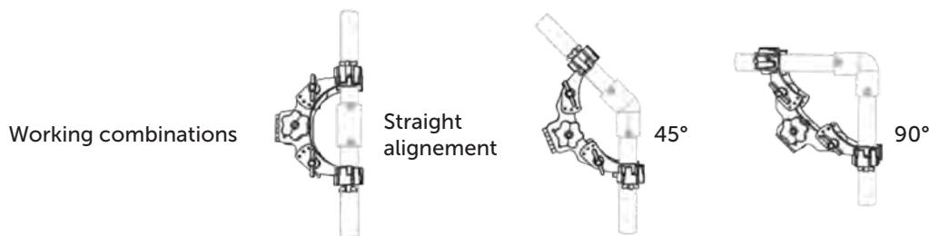
**9960-6318R** The Aligner Eco will align and support pipes from 63-180mm to facilitate welding of electrofusion couplers, 45° and 90° bends.
