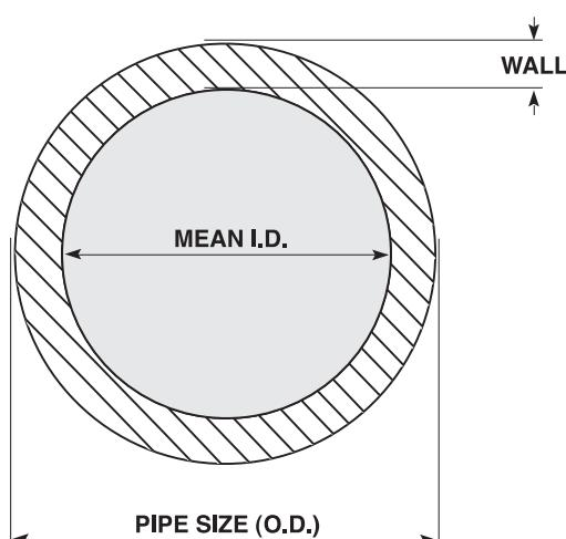
$$\text{SDR} = \text{OD} \div \text{WALL THICKNESS}$$
