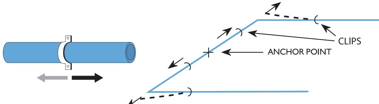
Free axial movement of pipework should be allowed with any form of support. Pipework should be able to move longitudinally without conflicting with elbows, tees, etc.
