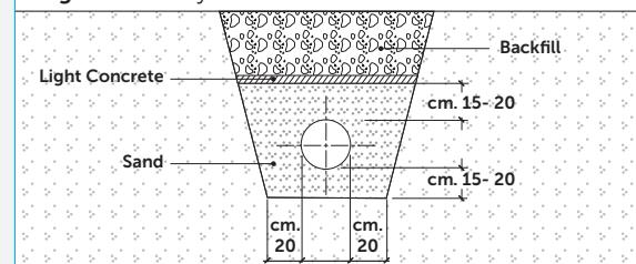
**Figure 9** Rigid Installation
