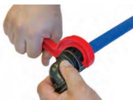
For sizes 40-63, use a nut wrench to tighten the nut a further half turn.
