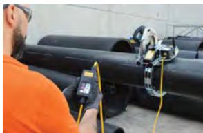
The saw orbital automatic movement is managed at a distance by the operator thanks to a joystick.
