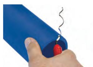
Use chamfer tool to remove sharp edge off the pipe and facilitate insertion through the O-Ring.
