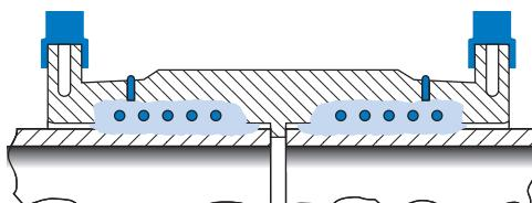
Melt pressure reaches optimum value at end of energising cycle. The pop up indicator appears to show fusion is complete.
