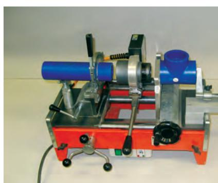
The bench mounted socket fusion welder is recommended for 90mm and 110mm, but is great for 63mm and smaller sizes. It provides mechanical advantage and consistency for the larger sizes.
