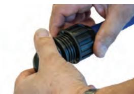
Firmly hand tighten the nut. Check witness mark.
