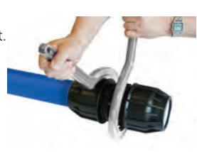
For sizes 75 -110mm use two nut wrenches to tighten the nut. Nut should be firmly tightened, but does not need to actually meet the external stop.
