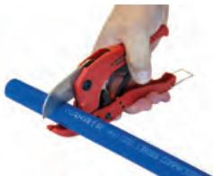
Cut pipe to length with pipe cutters for a clean swarf free finish.
