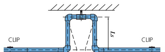
Typical expansion joint. Note fixed anchor point at centre of loop. No clips or fixings on legs. Clips on long run to allow for longitudinal expansion/contraction.
