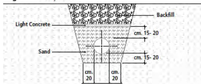
**Figure 3** Rigid Installation
