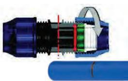
Undo the nut up to the last thread, do not remove the nut from the body. Insert the pipe through the nut into the fitting until it meets the stop.
