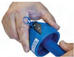
Use chamfer tool to remove sharp edge off the pipe and facilitate insertion through the O-Ring.
