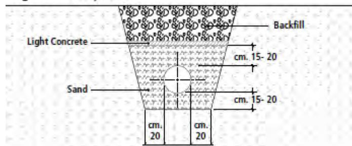
**Figure 3** Rigid Installation
