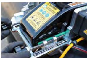
Intuitive and easy working range adjustment. The cutting process is performed directly at the jobsite after mounting the needed clamps according to the pipe diameter.
